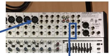
Next, take a 3.5mm to Phono plugs lead with ¼ inch mono adaptors and connect the ¼ inch plugs to subgroup outputs 1 and 2 (left and right) shown above. The 3.5mm plug connects to the microphone socket on the video camera.
