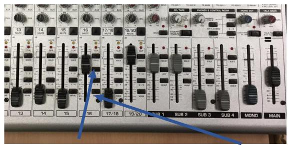
Make sure that the 1-2 button to the right of the channel 16 slider is pressed in, and Main is also pressed in.
